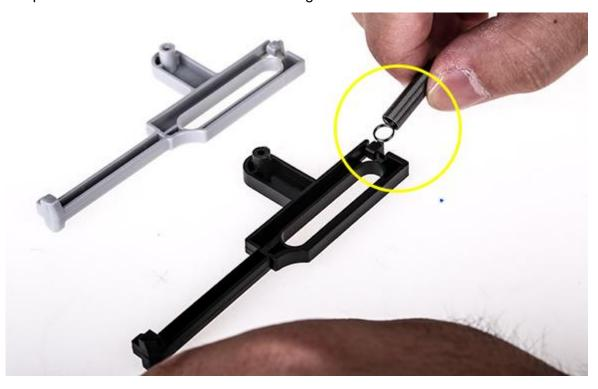
**Step 5:**Install the hammer module into the body.
