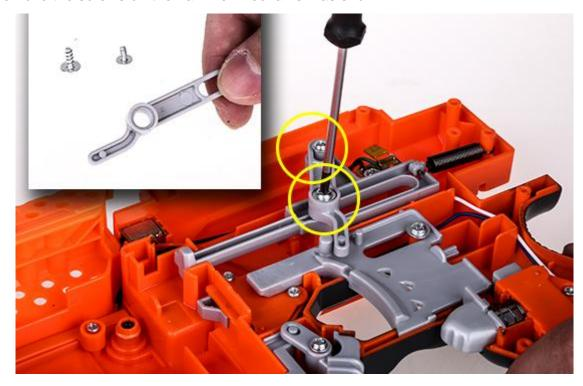
**Step 3:**Remove the spring coil and the module out of the body.
