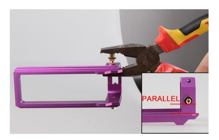
**Step 2:**Install the dart catcher into the bolt shed, insert the metal rod to secure the dart catcher in position.
