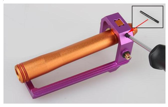
**Step 3:**Install the remain plunger tube, pump and catch back to the blaster body.
