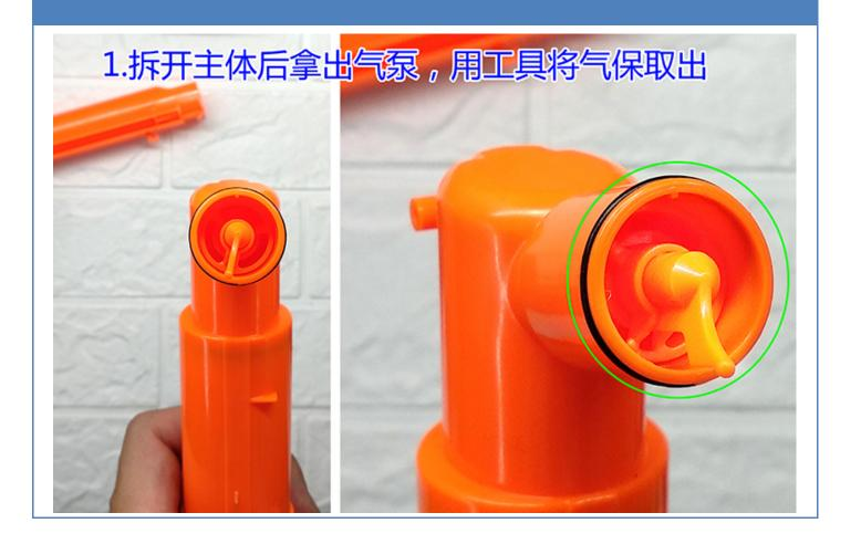
Refer to below picture, after removing the air restricker, the chamber shall be same as the picture.
