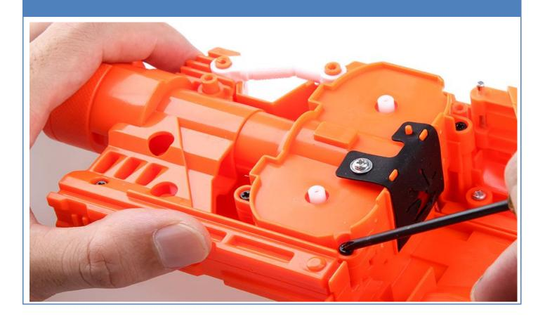
Remove the screws on the electric circuit module as shown, keep all the screw at safety place.
