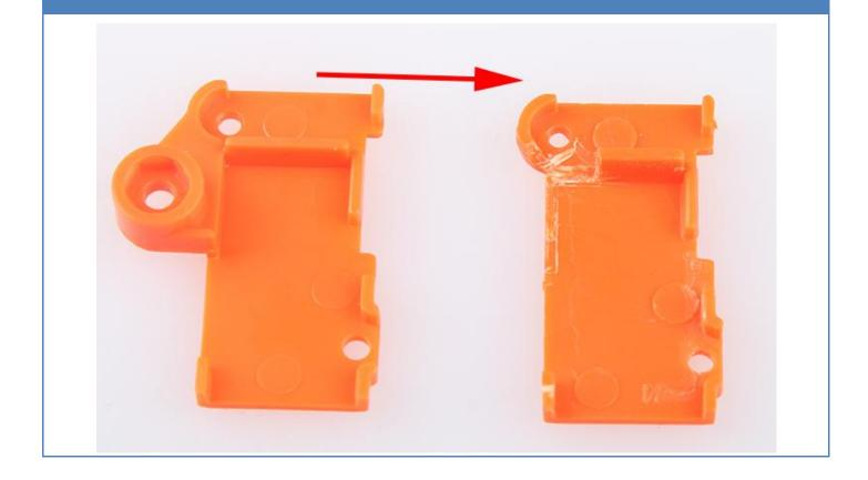
**Step 11** Trim the screw column under the on/off switch as shown.
