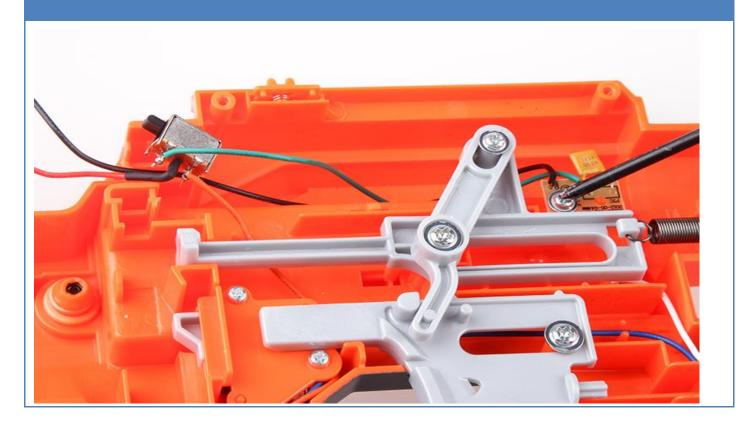
Remove the circuit on magazine switch. Please be reminded the protection on magazine in place would be removed.
