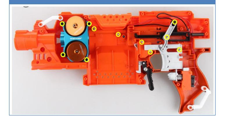
**Step 24** Install the front barrel tube to the flywheel cage and the front muzzle.
