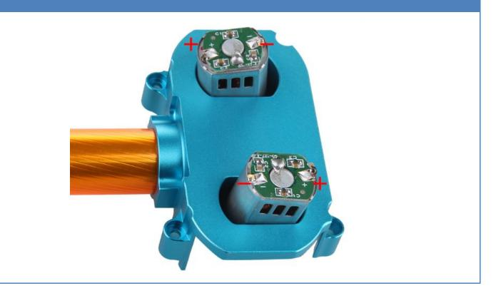
Fastern the screws on the cage to secure the motors in correct position.
