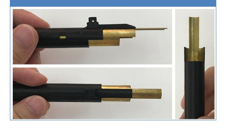
**Step 7:** Insert the bolt tube into the printed bolt and make it at correct position, contour exact the same. Apply small amount of instant glue make the bolt fix together, especially the tongue of the bolt
