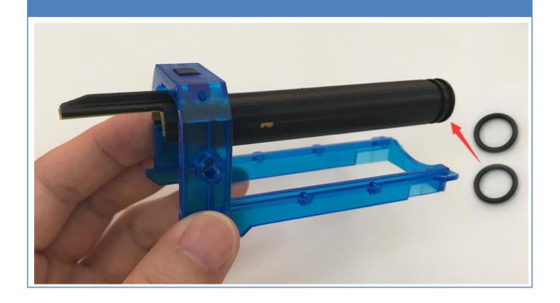
**Step 9:** Insert the barrel tube to the muzzle thought the printed fixture
