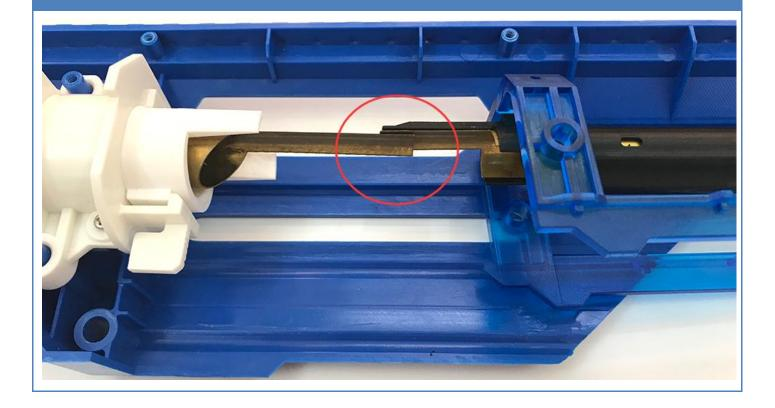
**Step 12:** Remove the plunger module and keep the chamber.
