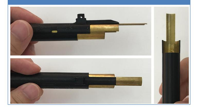
**Step 9:** Apply small amount of instant glue make the bolt fix together, especially the tongue of the bolt
