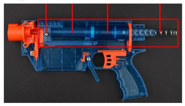
**Step 5:**Cover the blaster halves and insert the spring coil, apply force to push the whole spring coil stay inside and pushing the rear stock.
