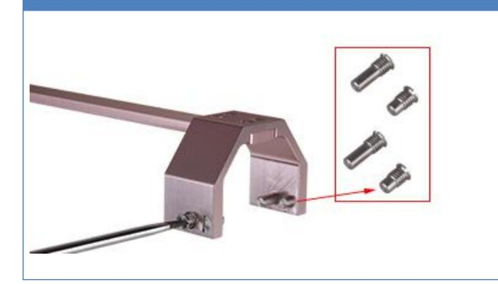
Step 7: Install the prime rod to the body. Match the screw to the boltshed and fasten the screws to connect the prime rod to the boltshed.
