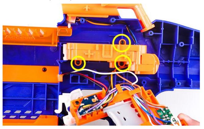
**Step 6:**Detach the hammer module, remove the screws (as shown) and carefully opening the housing.
