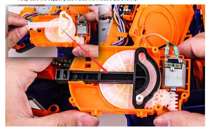
**Step 9:**Check carefully the shaft and teethes in correct position before closing the module (position as shown).
