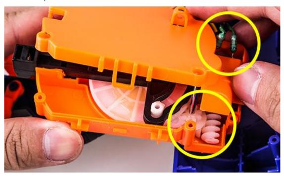
**Step 10:**Reverse action to assemble all the modules and screws into the body.
