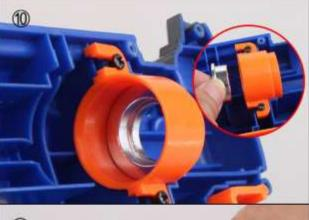
10) Install the metal cap to the spring stopper parts as shown.
