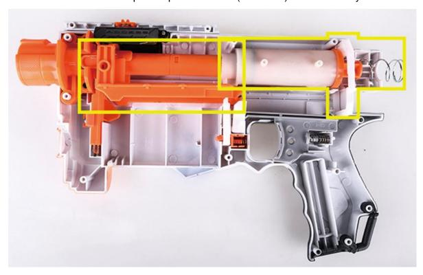
**Step 5:**Replace the rear plate spring coil with Worker MOD spring coil.
