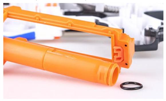
**Step 9:**Trim and polish the plastic part as show location, to ensure proper install the buffer piece.
