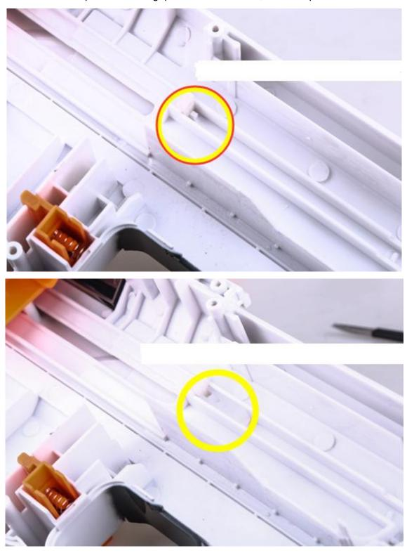
**Step 11:**Lubricate the O-ring and piston tube wall before assemble the module.
