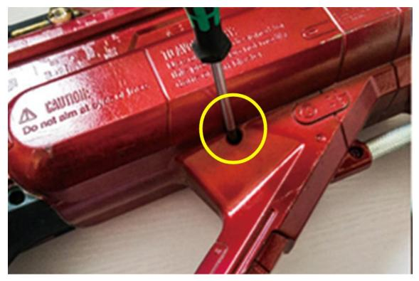
**Step 3:**Cut the sticker in the battery apartment, to ensure no hinder while dissemble the halves.
