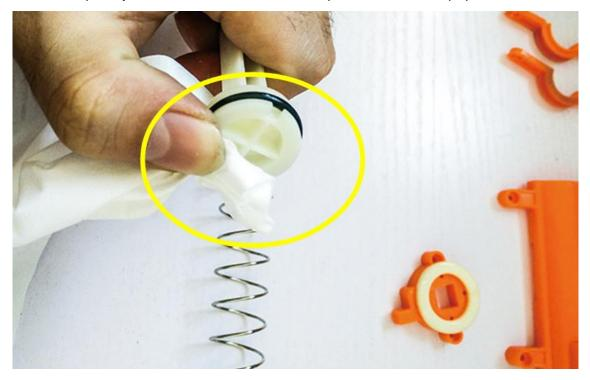
**Step 8:**Remove the rubber O-ring on the piston end.
