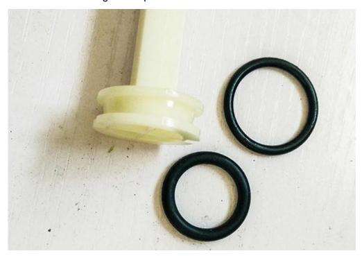
**Step 9:**Polish the piston end with fine sand paper, to ensure good adhesive strength of buffer pad.
