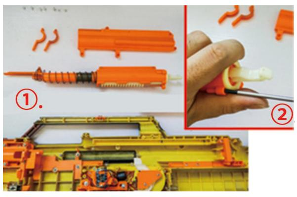
**Step 6:**Take out the spring coil and piston from the tube housing.
