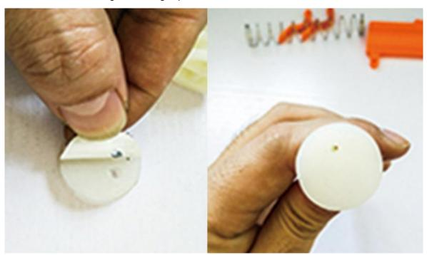
**Step 12:**Trim the buffer pad as the shape of piston end.
