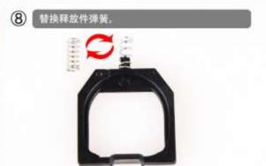
8) Replace the spring coil on the catch plate with given stronger spring coil.
