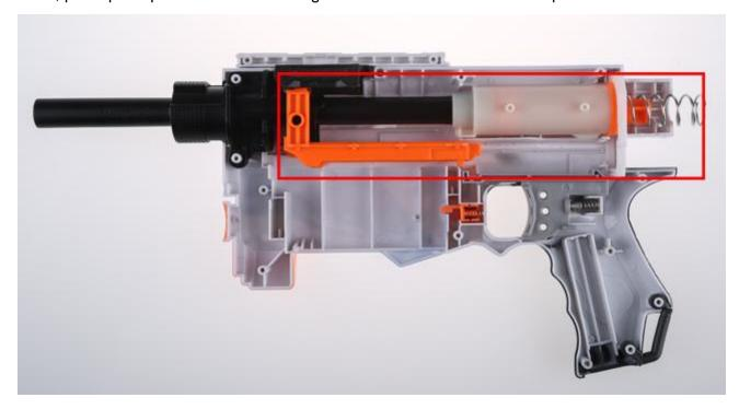
**Step 3:**Replace the connector on the dart loading mechanism part by brass cylinder connectors provided with the kit.
