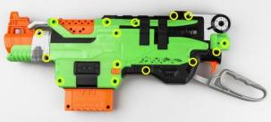
2) Remove all the screws on the blaster, open the shell and keep all the screw well.
