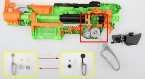
4) Locate the grip level module, replace the stock plastic level system with the metal gear and grip.
